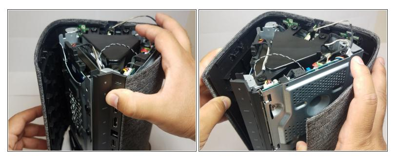
• Pry open the casing from the back of the IO panel, as shown in the pictures.
