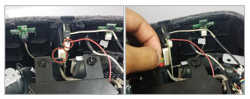
• Finally, remove the two cables circled in red from the front IO panel.
