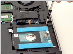
Use a PH1 screwdriver bit to remove the four M2.5x5 screws (2.4 mm) on the hard disk drive.
