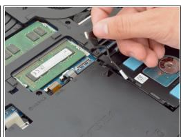
Gently lift the HDD cable to disconnect it from the laptop.
