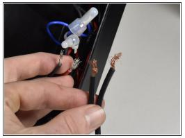
Untwist the two wires from each other and pull the zip tie off.
