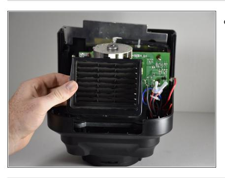
Grip the vent on either side and lift it straight in the upward direction.
