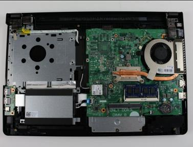
Gently pry the back cover from the opposite side of the battery to reveal the internal components.
