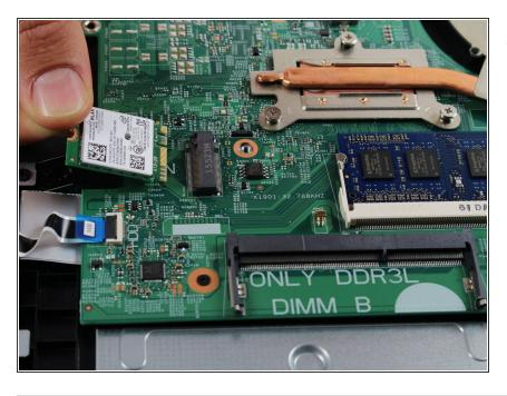
Gently pry the wireless card upward from the screw-side and pull outward toward the edge of the laptop to remove.
