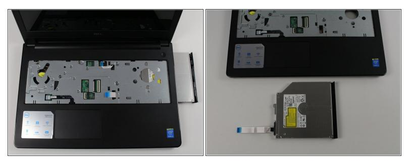
• Slide the optical drive out of the port on the right-side of the laptop.
