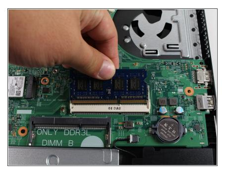
• Lift the RAM out of the memory port by first pulling forward, away from the port, and then upward.
