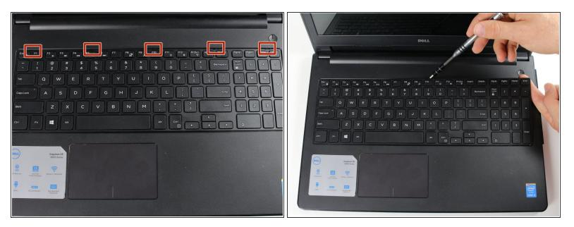
With the laptop open and facing upright, use the Spudger to pull at the notches shown in the image.
