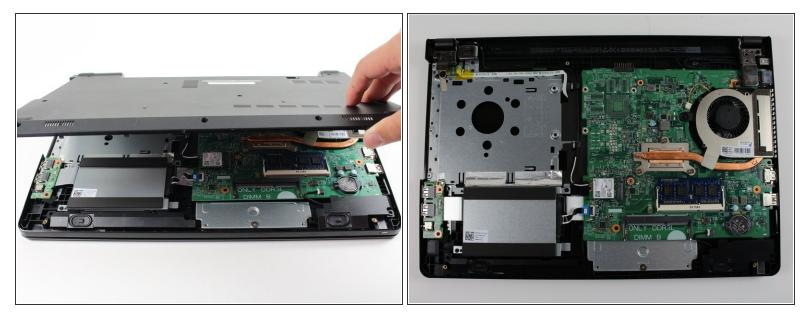
• Gently pry the back cover from the opposite side of the battery to reveal the internal components.
