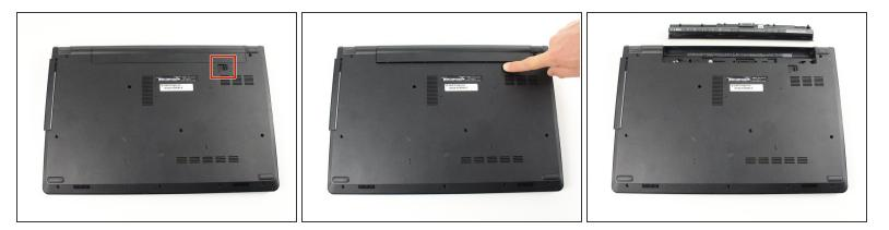
With the back of the laptop facing upright, press the switch shown to loosen the battery and remove it.
