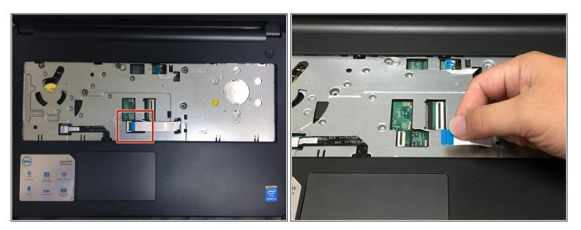
With the laptop facing upright - remove the ribbon cable from the optical drive by lifting the white release tab and gently pulling the cable away from the socket.
