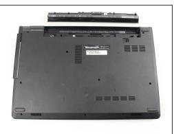
With the back of the laptop facing upright, press the switch shown to loosen the battery and remove it.
