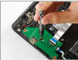
• Unscrew the two Phillips #00 4mm screws located on the USB chip.
