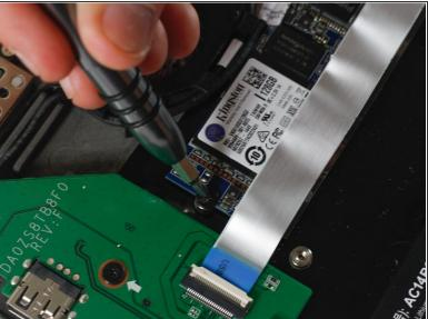
Remove the Phillips #00 4mm securing screw using your screwdriver.
