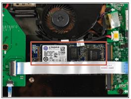
• Locate the hard drive, as shown to the left. This can be identified by its location underneath the cooling fan and above the ribbon cable (the long horizontal white strip).
