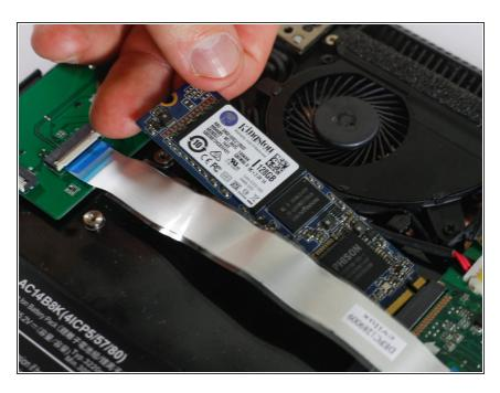
Remove the hard drive by pulling towards the side that was secured by the screw.
