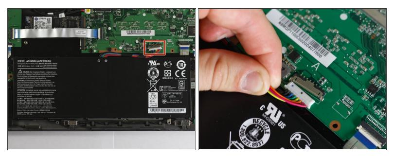
Disconnect the battery from the motherboard by simply pulling the wires down towards the battery until the adapter dislodges.
