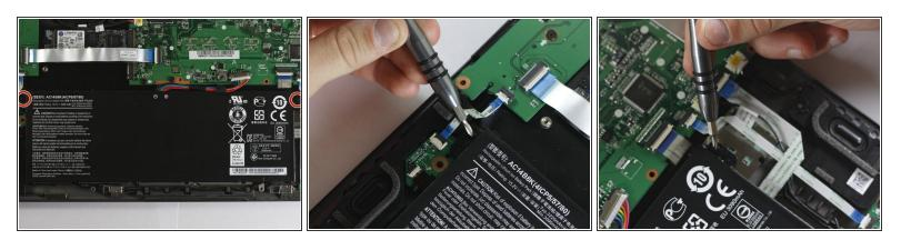
Remove the Phillips #00 5mm securing screws using your screwdriver.
