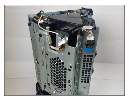
Locate a blue USB adapter on the left side of the hard disk compartment.
