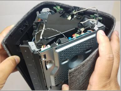
Pry open the casing from the back of the IO panel, as shown in the pictures.
