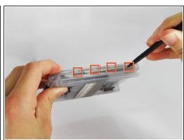
• Use the spudger to pry open the casing by applying pressure at 4 clips on both sides of the device.
