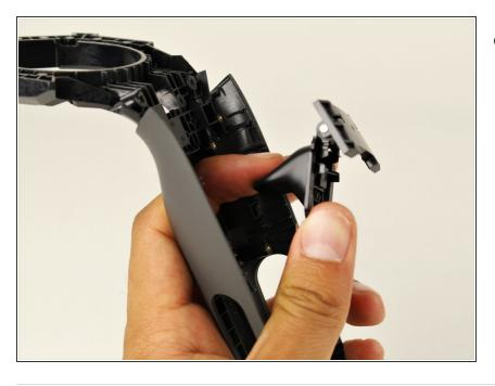
Push the trigger button in with your finger until it pops out of the front panel.
