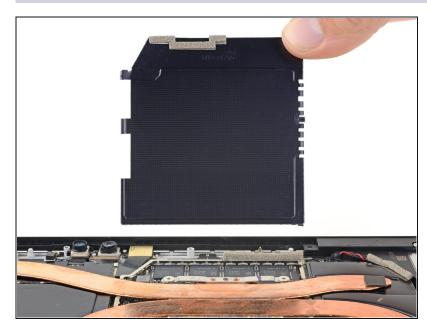
• Remove the heat sink shield.
