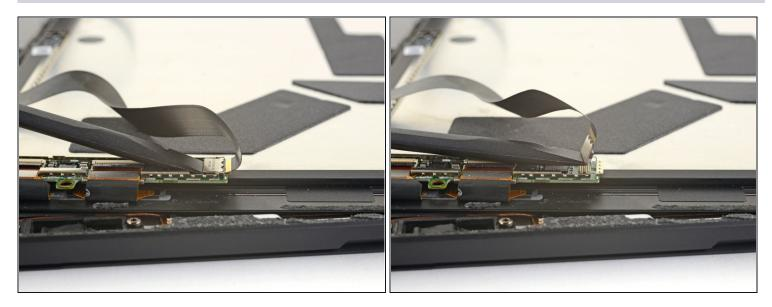
• Use the flat end of a spudger to pry the display interconnect cable straight up and out of its socket on the board.
