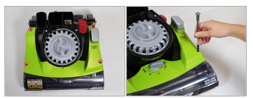
• Remove the four 20mm screws on the top of the vacuum head's cover using a JIS 1 screwdriver.
