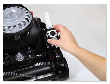
• Lift up on the belt latch assembly and remove it from the vacuum.
