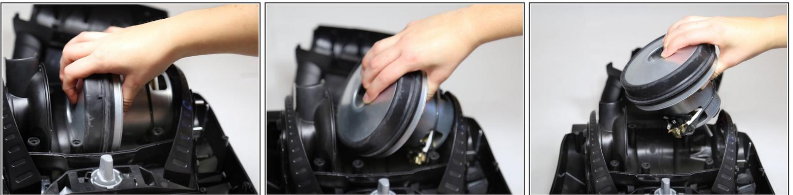
**i** There is a black wire that connects the cover to the motor. Be careful to keep this wire connected and undamaged while removing the motor.
