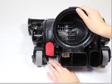
• Press the handle release pedal and rotate the motor cover downward until it is fully reclined.
