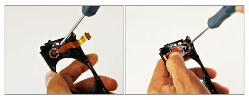
Use the T5 Torx head screwdriver to remove the two silver 4.2mm screws from the rear plastic cover of the menu button.
