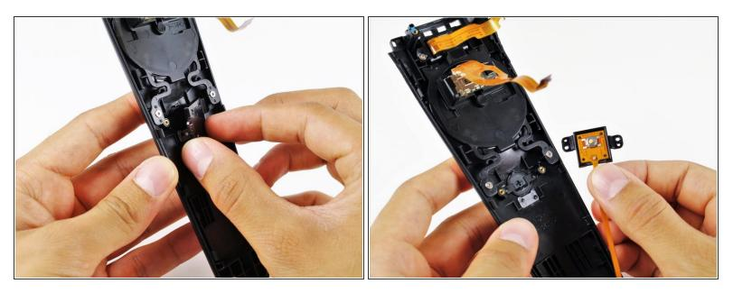
• Lift the plastic cover up and out of the front panel using your hand.
