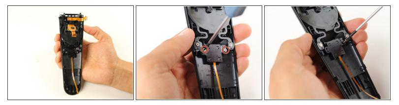
Use the T5 Torx head screwdriver to remove the two silver 4.2mm screws from rear plastic cover of the system button.
