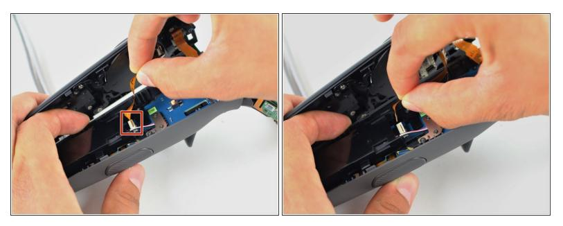
Disconnect the middle ribbon cable gently by pulling the ribbon cable up and away from the motherboard with two fingers.
