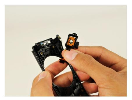
Lift the plastic cover up and out of the panel using your hand.
