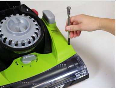
• Remove the four 20mm screws on the top of the vacuum head's cover using a JIS 1 screwdriver.
