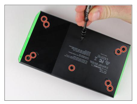
Remove the ten 6 mm screws using a T8 screwdriver.
