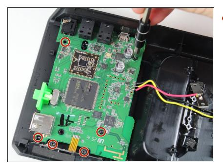
Remove the six 6mm screws using a T6 screwdriver.
