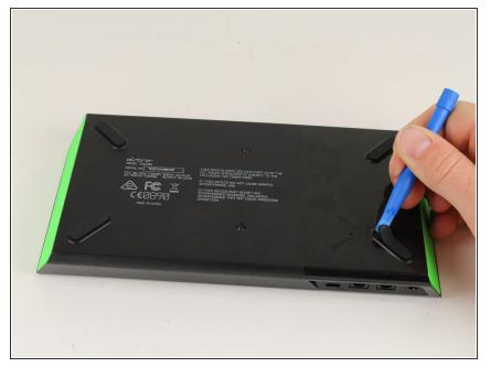
• Remove the four rubber feet from the bottom of the base station using the plastic opening tool.
