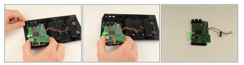
• Lift up the motherboard from the base station and pull it away from the device to remove it.
