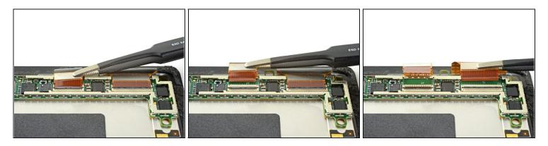
• Use <u>tweezers</u> to slide the display cables straight out of their sockets on the display board.
