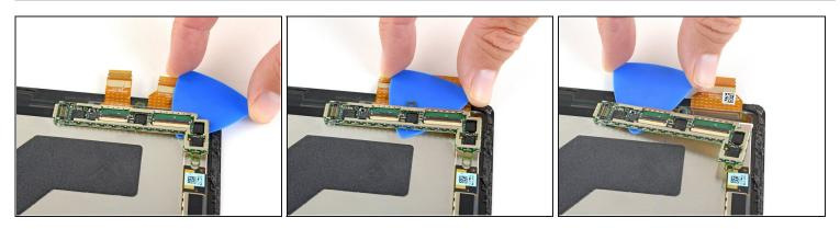
• Slide an opening pick under the display board to separate the adhesive holding it onto the back of the screen.
