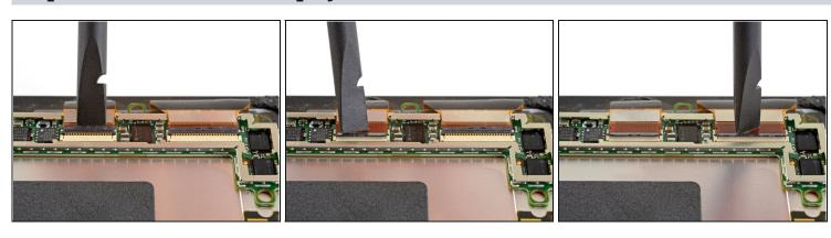
• Use a spudger to flip up the small locking flaps on the display cable ZIF connectors.
