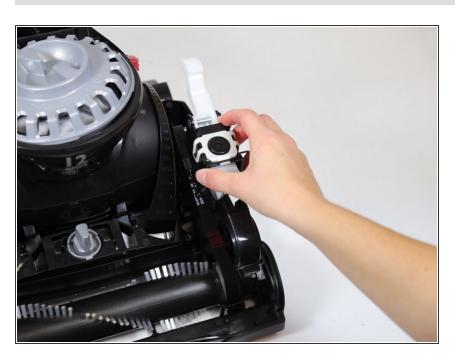
Lift up on the belt latch assembly and remove it from the vacuum. To reassemble your device, follow these instructions in reverse order.
