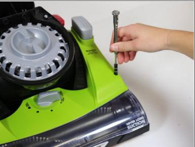
• Remove the four 20mm screws on the top of the vacuum head's cover using a JIS 1 screwdriver.
