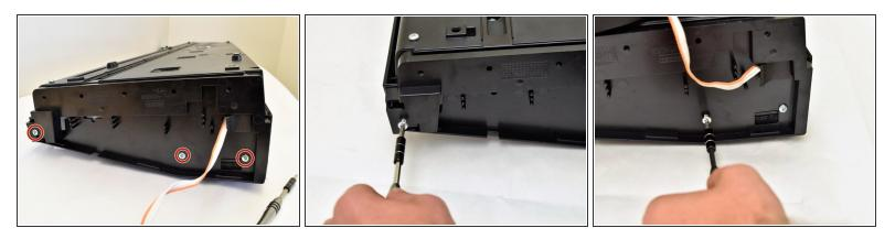
Remove the three silver 10mm screws with a J1 screwdriver on the bottom half of the innermost side panel of the device.
