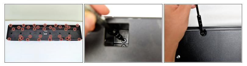
• Remove the 36 silver 10mm J head screws with a J1 screwdriver from the back panel.
