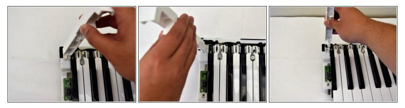
• Wiggle the white key from side to side and pull up to detach it from the rest of the board.
