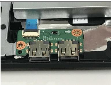
Remove the cable (look for the one with a blue tag reading "USB") very carefully as it is fragile by using the opening tool.
