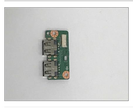
The USB ports should now be able to be removed from the laptop, carefully.
