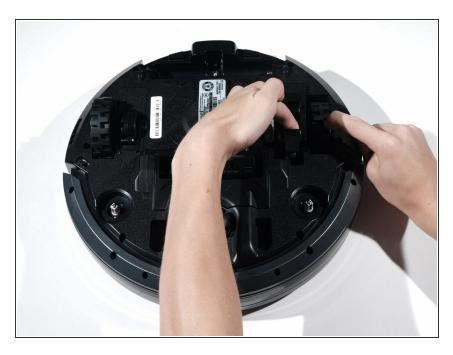
Put one finger on the wheel and the other under the access cover.
