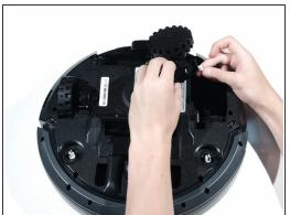
Remove the spring and carefully pull the wires out to disconnect the wheel from the socket.
