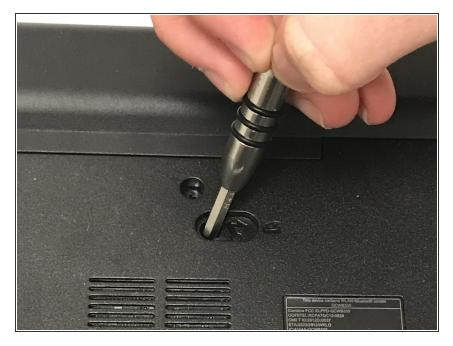
Below the battery, slightly to the right of the center of the laptop will be a switch indented into the case. This is the battery release.
