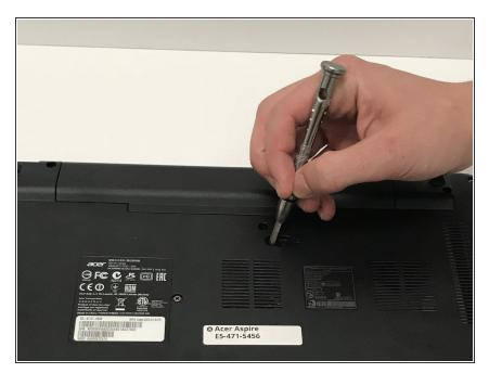
• To remove the battery flip the laptop over and locate the battery.
