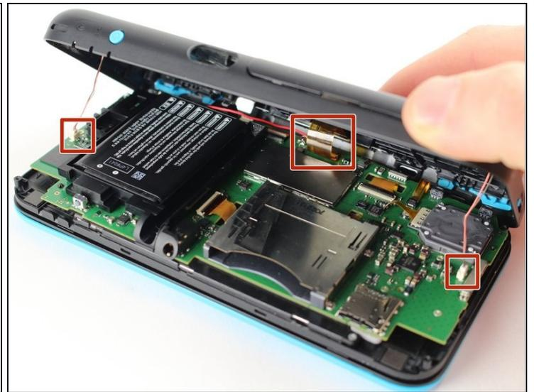
**⚠** Be careful when separating the bottom panel from the front casing to avoid breaking the three cables connected to the motherboard (two on each side and one in the rear).
