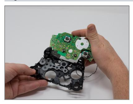
To avoid disconnecting the wires connected to the motherboard, lift the mother board away from the plastic frame as if opening a laptop.
