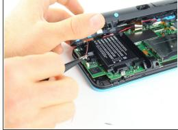
Using tweezers, disconnect the two cables that connect the rear buttons on either side to the motherboard by gently pulling them upwards.
