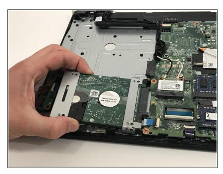
Slowly lift the hard drive with its corresponding securing plates up and out of its housing unplugging it from the motherboard.
