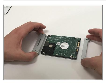
Once completely removed, separate the hard drive from the securing plates.
