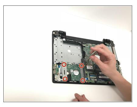
Locate the hard drive at the bottom left corner of the laptop. On the silver plate securing the hard drive,
