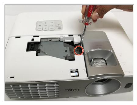
Using a Phillips #1 (PH1) screwdriver, loosen and remove the single 2.5 mm Phillips #1 screw that secures the lamp housing to the projector.
