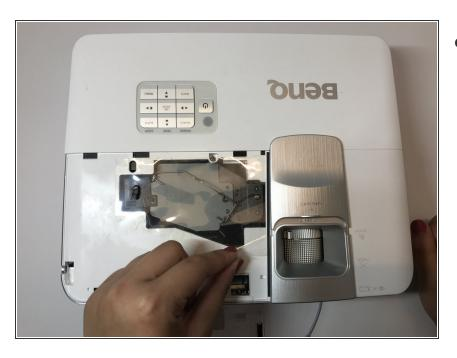
Carefully peel off the adhesive film covering the lamp housing.
