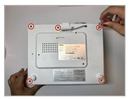
Turn the projector over (upside down) and remove the five 9.5 mm Philips #1 (PH1) screws that hold the projector together to its bottom cover.
