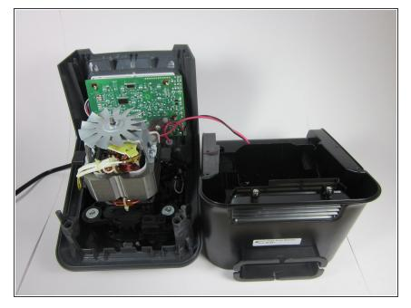
This completes the disassembly of the main body of the blender so you can continue to perform replacements on the internal parts.
