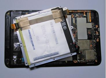
• Remove unscrewed battery tray from main frame.
