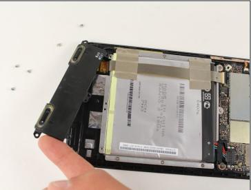
• Remove screws (2.6mm) connecting speaker to hard frame with Phillips head screw driver (PH000).
