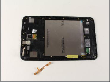
• Peel off button sensors off the side of the hard frame.
