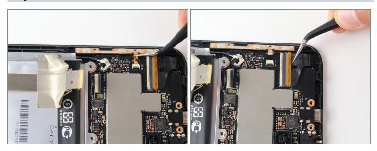
Remove display and button connections from motherboard using metal tweezers.
