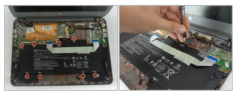
• Remove the eight 4mm screws holding the battery in place using the Phillips #00 screwdriver.
