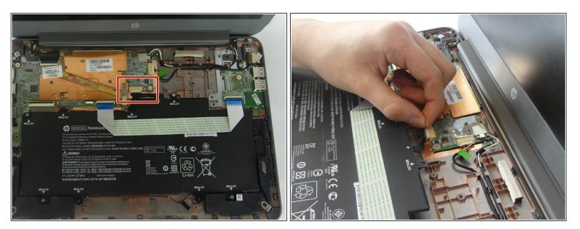
Unhook the battery's power connector from the motherboard.
