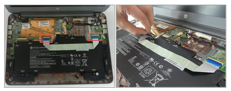
Remove the ribbon cable that runs over the battery by lifting up the plastic latches and pulling the cable away.
