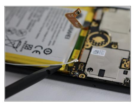
Use a spudger to gently pry off the small antenna cable on the right side of the motherboard.
