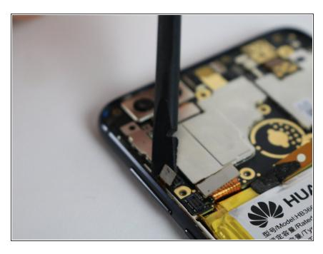
Use a spudger to gently pry off the small connection on the far left edge of the motherboard.
