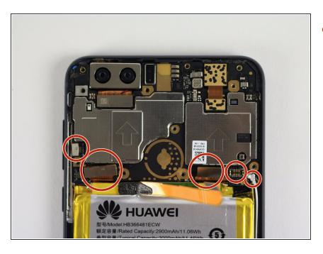
In the following steps you will disconnect the five connectors circled in red holding the motherboard in place.
