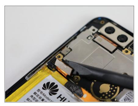
Using a spudger, gently pry up the connector near the left edge of the motherboard.
