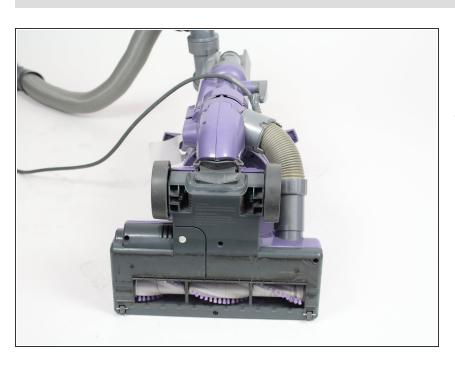
Lay down the vacuum to access the bottom panel of the roller brush compartment.
