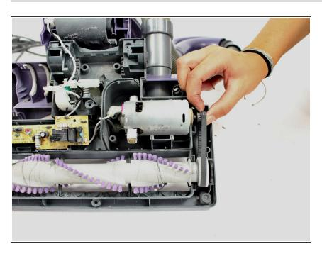
Lift up and then pull the roller belt off of the roller brush and the motor to remove it.
