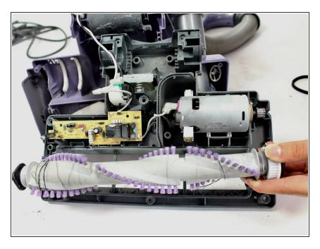
Take out the roller brush by lifting it out of its tray.
