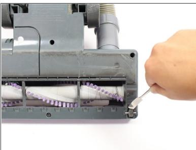
• Using the metal spudger, pry the two small wheels located at the two bottom corners of the vacuum to remove them.
