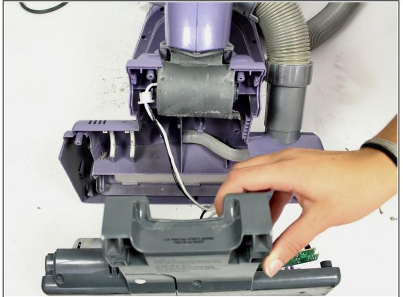
**⚠** Perform the next step slowly and carefully so the wiring connecting the motherboard to the rest of the vacuum is not broken.
