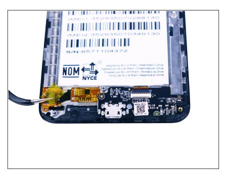
Remove the transparent tape covering one of the ribbon connectors using the tweezers.
