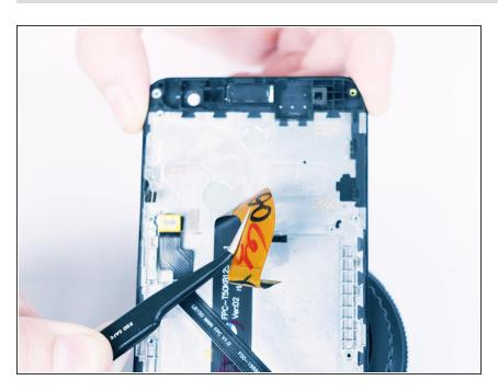
Take off the sticker and the ribbon cables glued to the back of the screen.
