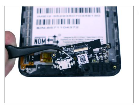
Lift the daughterboard from the frame using the plastic opening tool.
