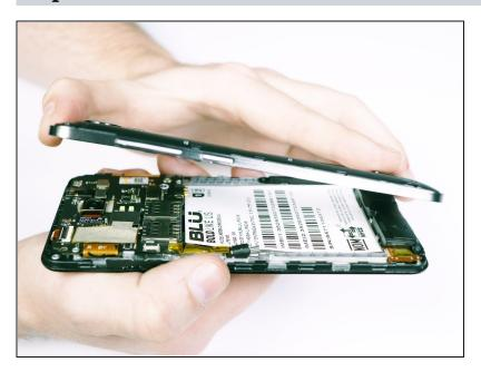
Once all the clips have been released, pull back the frame and set it aside.
