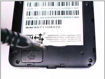
• Use the Phillips #00 (1.5mm) bit to undo the (9) screws from the back of the device.
