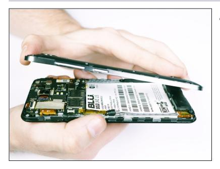
• Once all the clips have been released, lift the frame and set it aside.
