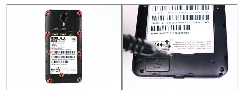
• Use the Phillips #00 bit to undo the nine 1.5mm screws from the back of the device.
