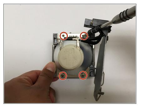
With a Philips #0 (PH0) screwdriver, remove the four screws that secure the bulb to the housing unit.
