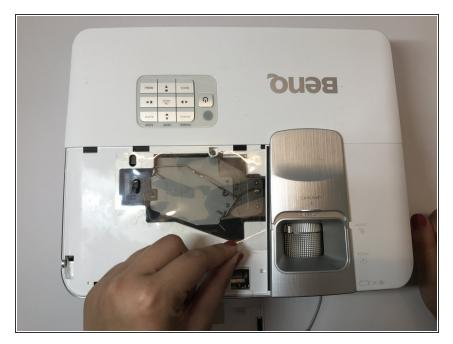
• Carefully peel off the adhesive film covering the lamp housing.
