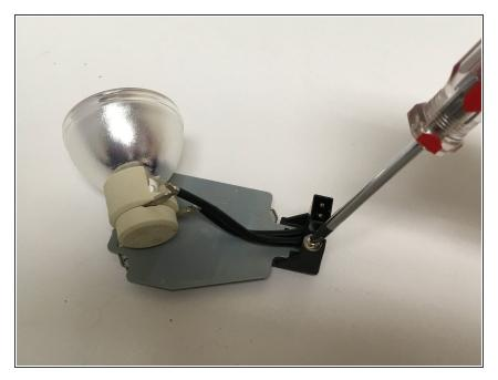
• Using a Philips#1 (PH1) screwdriver, remove the 2.5 mm Phillips #1 screw that secures the wires to the detach bulb.
