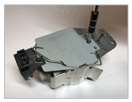
Using a 2.5mm Hex key, remove the top portion that contains the handle. This portion is also attached to the bulb housing.
