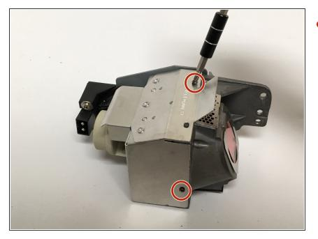
Using a Philips #0 (PH0) screwdriver, remove the two screws holding the metal case of the lamp housing.
