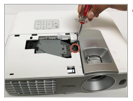
Using a Phillips #1 (PH1) screwdriver, loosen and remove the single 2.5 mm Phillips #1 screw that secures the lamp housing to the projector.
