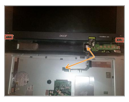
Flip the laptop over again, and open it just about all of the way, so that you can access the screws securing the hinges. Remove the screws.
