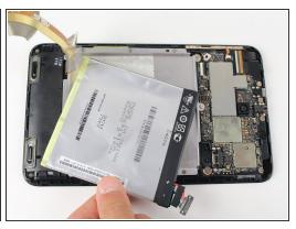
Wedge the flat end of a spudger or plastic opening tool under the battery to free the battery form any adhesives.
