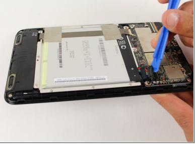
Locate the black bundle connector on the back of the device. Gently slide the plastic tool underneath the black bundle cable connector towards the battery until it comes off.
