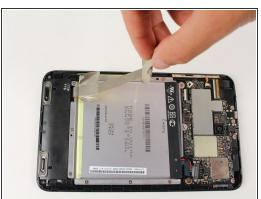
Using the plastic opener tool, carefully remove the ZIF connectors that is covering the battery.
