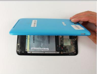
Separate the front and back by prying in between the two with a plastic opening tool.
