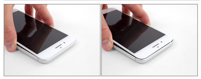
Slide the display assembly slightly down (away from the top edge of the phone) to disengage the clips holding it to the rear case.
