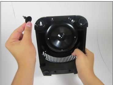
Pull the damaged suction cup off of its pit.
