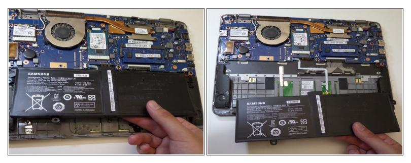
• Lift the battery up at an angle to disconnect the battery from the motherboard, then pull it away from the laptop.
