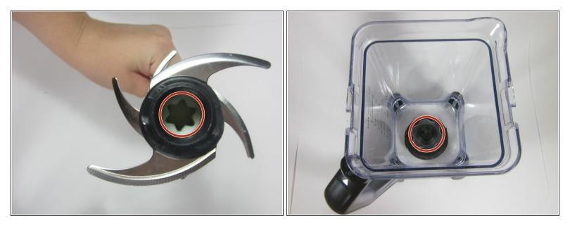
• Carefully pick up the new blade and match the bottom star shaped opening to the star shaped protrusion from the blender.
